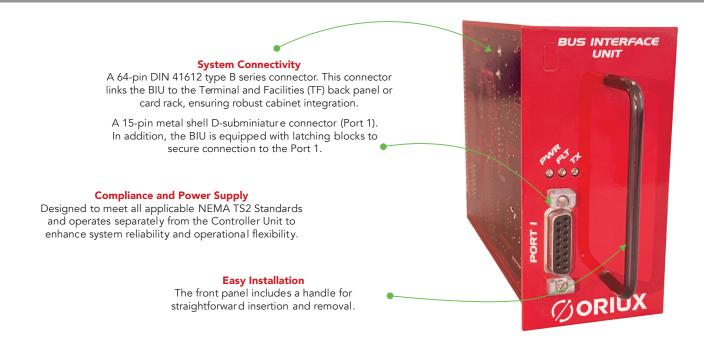
Oriux BIU is designed to meet all applicable NEMA TS2 Standards and operates separately from the Controller Unit to enhance system reliability and operational flexibility.
